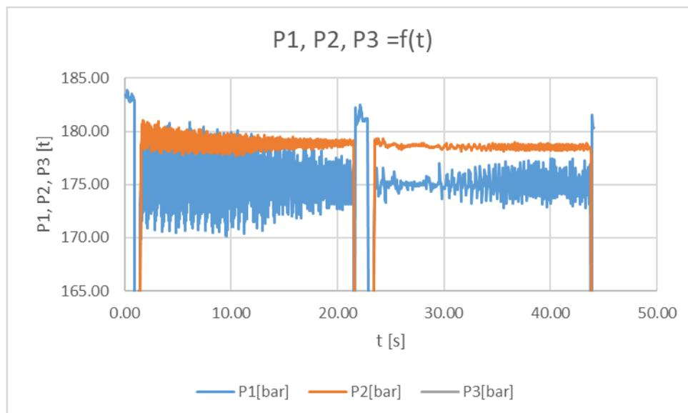
**Fig. 7.** Detail: time-variation of pressures P1 and P2
