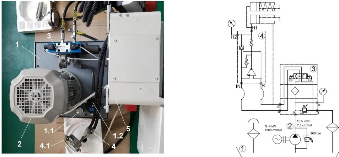
**Fig. 3.** Low-pressure pumping unit equipped with minibooster:
