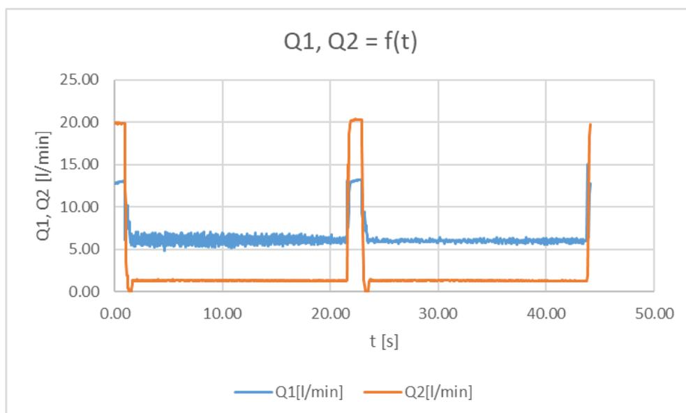
**Fig. 9.** Time-variation of flow rates Q1 and Q2
